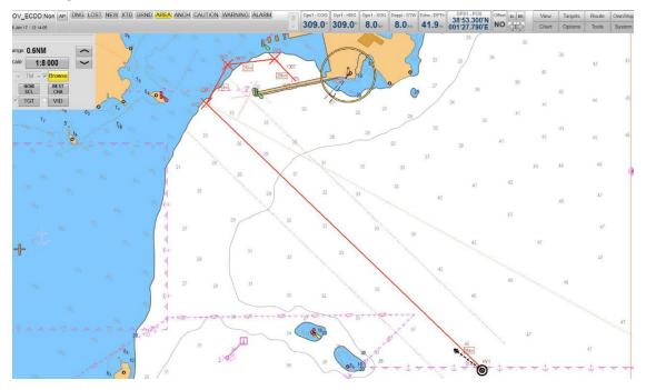
Once the route has been accurately drown, arriving to the berth, it is not possible to validate, due that on some waypoints the route has "bad geometry", meaning that turning radius results too tight. But, what is the minimum Azi-pod turning radius? Obviously, even the concept of "bad geometry" has no sense in this case.
