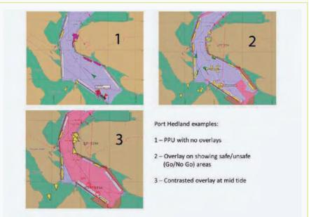
Figure 6 Actual PPU displays with overlays on/off and differing tidal conditions
