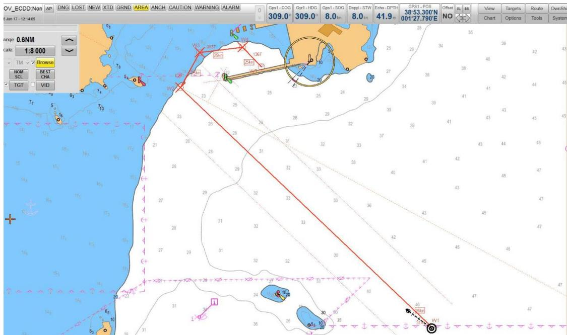
Once the route has been accurately drawn, arriving to the berth, it is not possible to validate, due that on some waypoints the route has “bad geometry”, meaning that turning radius results too tight. But, what is the minimum Azi-pod turning radius? Obviously, even the concept of “bad geometry” has no sense in this case.
